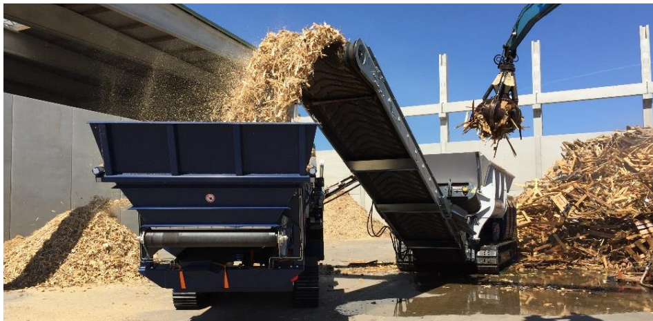
2 breakwaters of performance class 50t/h with starscreen 2-tb17
